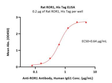
Immobilized Rat ROR1, His Tag (Cat. No. RO1-R5221) at 2  $\mu$ g/mL (100  $\mu$ L/well) can bind Anti-ROR1 Antibody, Human IgG1 with a linear range of 0.078-1.25  $\mu$ g/mL (QC tested).
