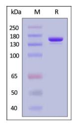
The gel was stained with Coomassie Blue. The purity of the protein is greater than 95% (With <u>Star Ribbon Pre-stained Protein Marker</u>).
