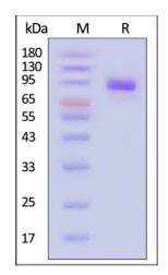
Human ErbB3, His Tag on SDS-PAGE under reducing (R) condition. The gel was stained with Coomassie Blue. The purity of the protein is greater than 95%.
