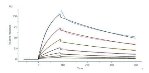
Anti-CCR7 Antibody, Human IgG1 captured on Protein A Chip can bind Human CCR7 Full Length Protein, His,Flag Tag (Cat. No. CC7-H52D3) with an affinity constant of 121 nM as determined in a SPR assay (in presence of DDM and CHS) (Biacore 8K) (Routinely tested).
