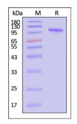
Human Cadherin-6 Protein, Fc Tag on SDS-PAGE under reducing (R) condition. The gel was stained with Coomassie Blue. The purity of the protein is greater than 90% (With <u>Star Ribbon Pre-stained Protein Marker</u>).
