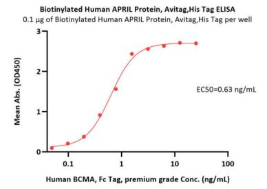
Immobilized Biotinylated Human APRIL Protein, Avitag,His Tag (Cat. No. APL-H82Q8) at 1  $\mu$ g/mL (100  $\mu$ L/well) on streptavidin (Cat. No. STN-N5116) precoated (0.5  $\mu$ g/well) plate can bind Human BCMA, Fc Tag, premium grade (Cat. No. BC7-H5254) with a linear range of 0.1-2  $\eta$ g/mL (QC tested).
