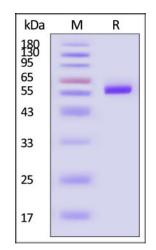
Biotinylated Human APRIL Protein, Avitag, His Tag on SDS-PAGE under reducing (R) condition. The gel was stained with Coomassie Blue. The purity of the protein is greater than 90% (With <u>Star Ribbon Pre-stained Protein Marker</u>).
