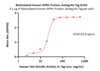
Immobilized Biotinylated Human APRIL Protein, Avitag,His Tag (Cat. No. APL-H82Q8) at 1  $\mu$ g/mL (100  $\mu$ L/well) on streptavidin (Cat. No. STN-N5116) precoated (0.5  $\mu$ g/well) plate can bind Human TACI (R119A, R122A), Fc Tag (Cat. No. TAI-H5253) with a linear range of 2-39 ng/mL (Routinely tested).
